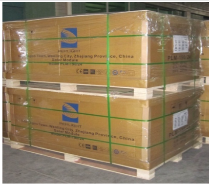
1. Stack two pallets, strapping, stretch film protection.
